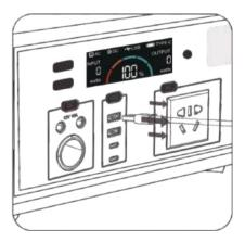
When finish using. Please pull off the plug and turn off the device.
