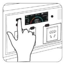
1 Long press 3 seconds of turn on/off switch to turn on the devices. LCD screen will turned on.
